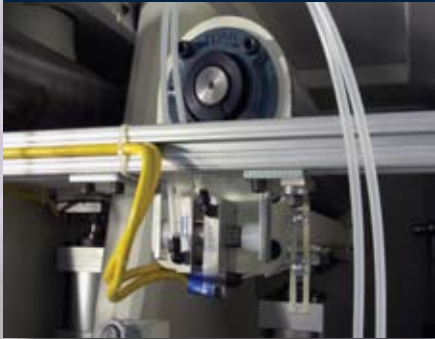
Self-aligning abrasive belt tracking system.
