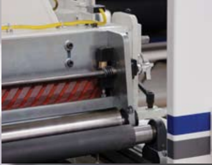
Adjustable platen with helical worm gear design.
