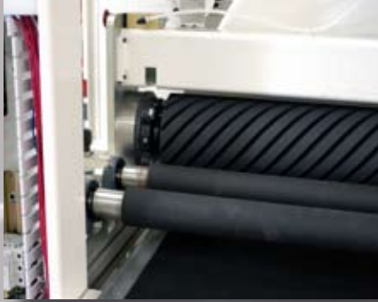
2 Heavy duty spring-loaded pinch rollers.
