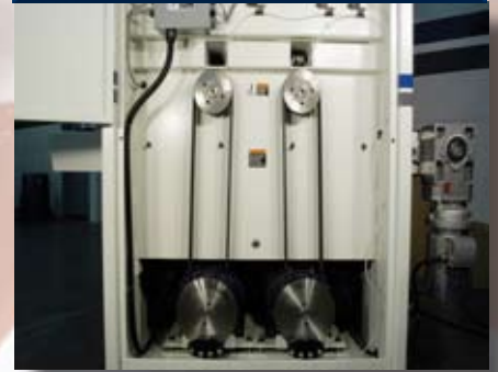
Individual TEFC drive motors with disc brake & pneumatic caliper.
